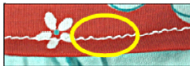
Poor Stitch Balance – Too Loose
