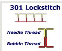
For 301 lockstitch seams, we generally recommend using the same needle thread size as the bobbin thread size in the seam. Why? Because *"a chain is only as strong as its weakest link."* If a smaller, weaker thread is used in the bobbin, then the seam will only be as strong as the bobbin thread. This is particularly true with lockstitch seams because of the way the needle and bobbin threads are interlocked together.
